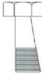
For holes drilled crooked
