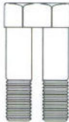
Binocular bolt for double drilled holes
