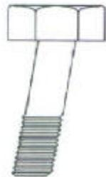
For holes which are mis-aligned
